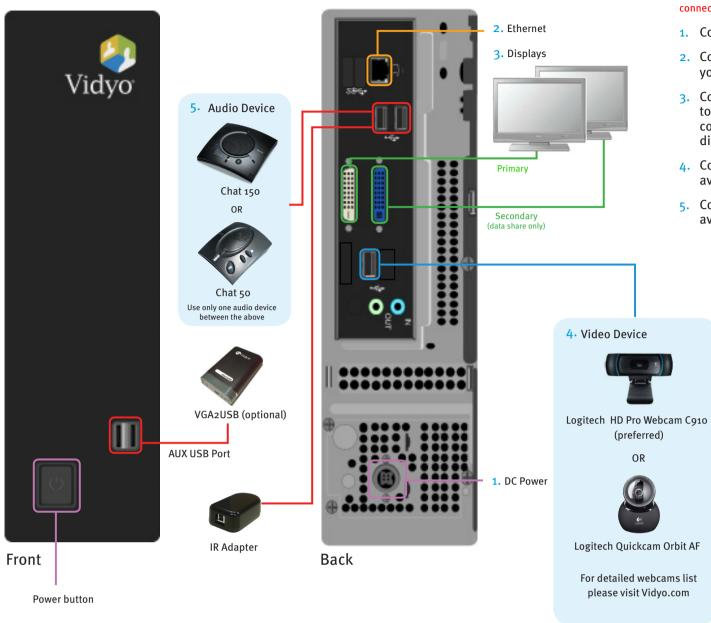
Do not power on HD-50 until the display(s) and camera are fully connected and powered on.
